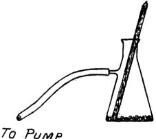
The authors while working on sulfonic acid derivatives devised the following simple apparatus:
